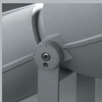
The angle adjustment - Locking teeth providing 10° adjustment intervals - Angle lock is available
